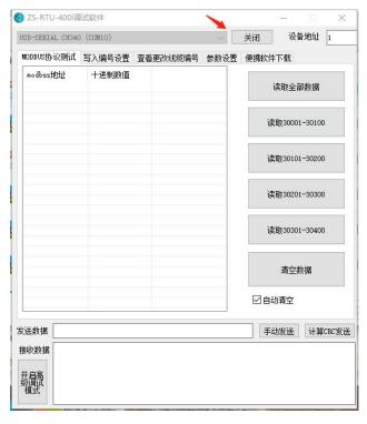
Fill in the device address in the upper right corner (default is 1)
